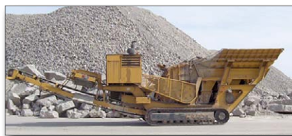
Figure 6. Crushed concrete stockpile and crusher
