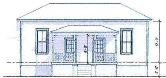
EAST/FRONT ELEVATION (new roof, columns, railings)
